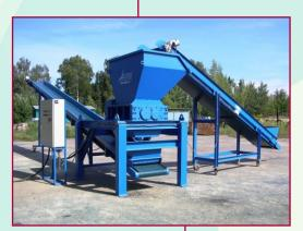
The operation of the shredder is checked by the reverse automatics, switching the shredder off in case of an overload and performing the reverse motion and switching the shredder to the shredding regime again. The automatics also secures the continual starting of the shredder and a possible starting of the input and output conveyers.
